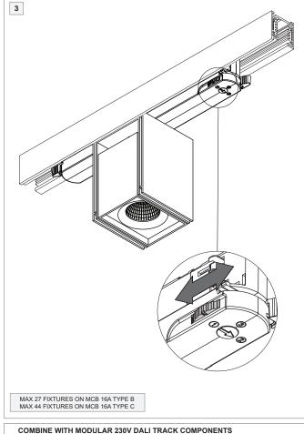
Consult Modular Lighting Instruments website or catalogue for overview track components. Fixture is also compatible with following track systems
