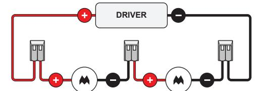
Always use a serial connection for multiple luminaires on a single driver!
