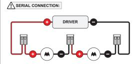
Always use a serial connection for multiple luminaires on a single driver! Only use luminaires with the same input ratings!
