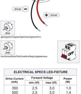
For serial connection, respect polarity! Not suited for connection to mains voltage. Combine with a Modular LED-driver.
