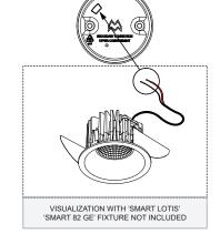
Connect fixture and close tube cover (re-use included toothed washers & screws)
