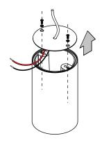
Disconnect fixture connectors and pull wires through opening
