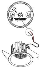
Disconnect fixture connectors and pull wires through opening
