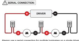
Always use a serial connection for multiple luminaires on a single driver! Only use luminaires with the same input ratings!
