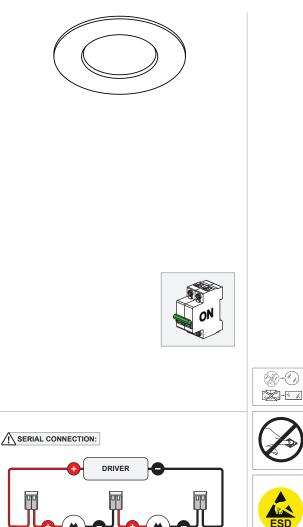
Always use a serial connection for multiple luminaires on a single driver! Only use luminaires with the same input ratings!
